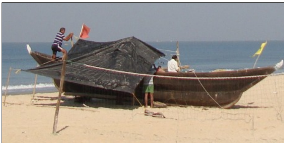
Figure 16 Damaged pirogue is traditionally beached bow-first. The crew erect a canopy to shade the boatbuilder. Fish Road. Author.
