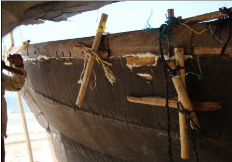
Figure 15 Despite use of scrap cords, close-set Spanish windlasses inboard and out exert pressure sufficient to bend a plank without steaming. Fish Road. Author.
