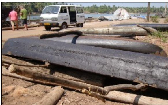
Figure 2. Monoxylous craft used on Goa's rivers. They are so heavily coated in dikh that sewn portions are difficult to detect: a) upturned with booms still attached. Assolna; b) under repair on the slip at Cavelossim. Author.
