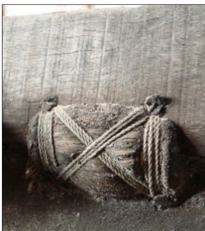
Figure 10. a) wedged stitch pad. Colva; b) narrow sheer strake with carved thole and thole-pin wear, flanked by paired padded stitches. Benaulim. Author.
