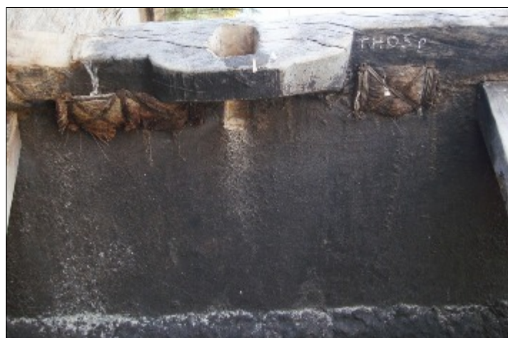
Figure 10. a) wedged stitch pad. Colva; b) narrow sheer strake with carved thole and thole-pin wear, flanked by paired padded stitches. Benaulim. Author.
